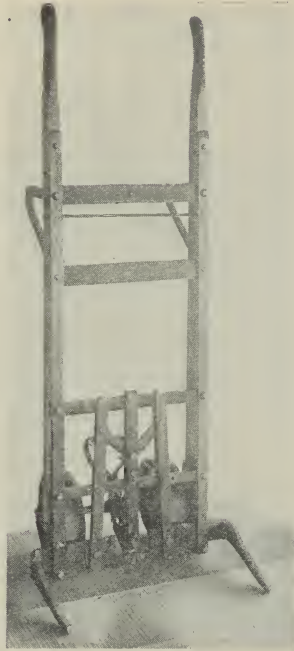
Fig. 7.—Warehouse truck, “clamp type.” The jaws which carry the load are opened and closed by means of foot levers.
